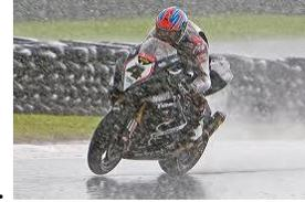
through those turns so quickly and effortlessly? It is smoothness. Your motorcycle has many dynamics, which change when you accelerate, brake, lean and stop. You may not feel it, but the chassis is shifting and the tire contact patches are transitioning. You want these transitions to be as smooth as possible, especially in the rain.
